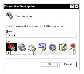
**4)** Next, *Hyper Terminal* needs to know how to "talk" to the CM16a. This selection depends on which port on your PC the null-modem cable is connected.
